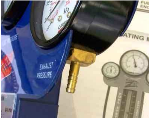
Vacuum gauge and exhaust pressure gauges have barbed nipples for a secure sample hose fit.
